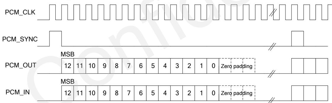
**Figure 31: Short Synchronization & Zero Padding Diagram**
